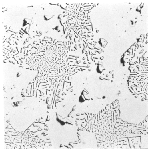
Figure 5 Optical micrograph of the sodium-modified Sb-Ge eutectic directionally solidified at 18 \text{ mm h}^{-1} . 0.8 wt% (4 at%) sodium added ( \times 96 ).
